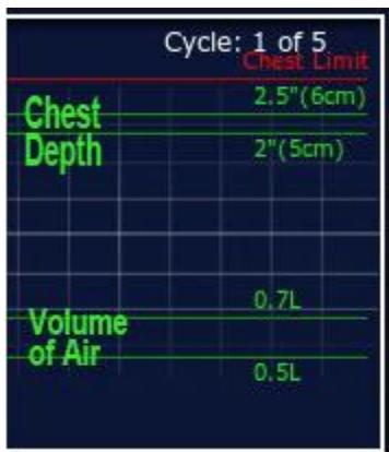
The two green horizontal lines on the right across the display, show the target depth of the compression. Push the chest until the bar goes between these two green lines.
